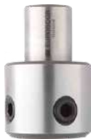
Adapter Weldon | 25 mm Shank: 19.05 mm (3/4") Weldon Extension length: 25 mm External dia: ø 35 mm
