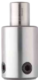
Adapter Weldon | 50 mm Shank: 19.05 mm (3/4") Weldon Extension length: 50 mm External dia: ø 35 mm
